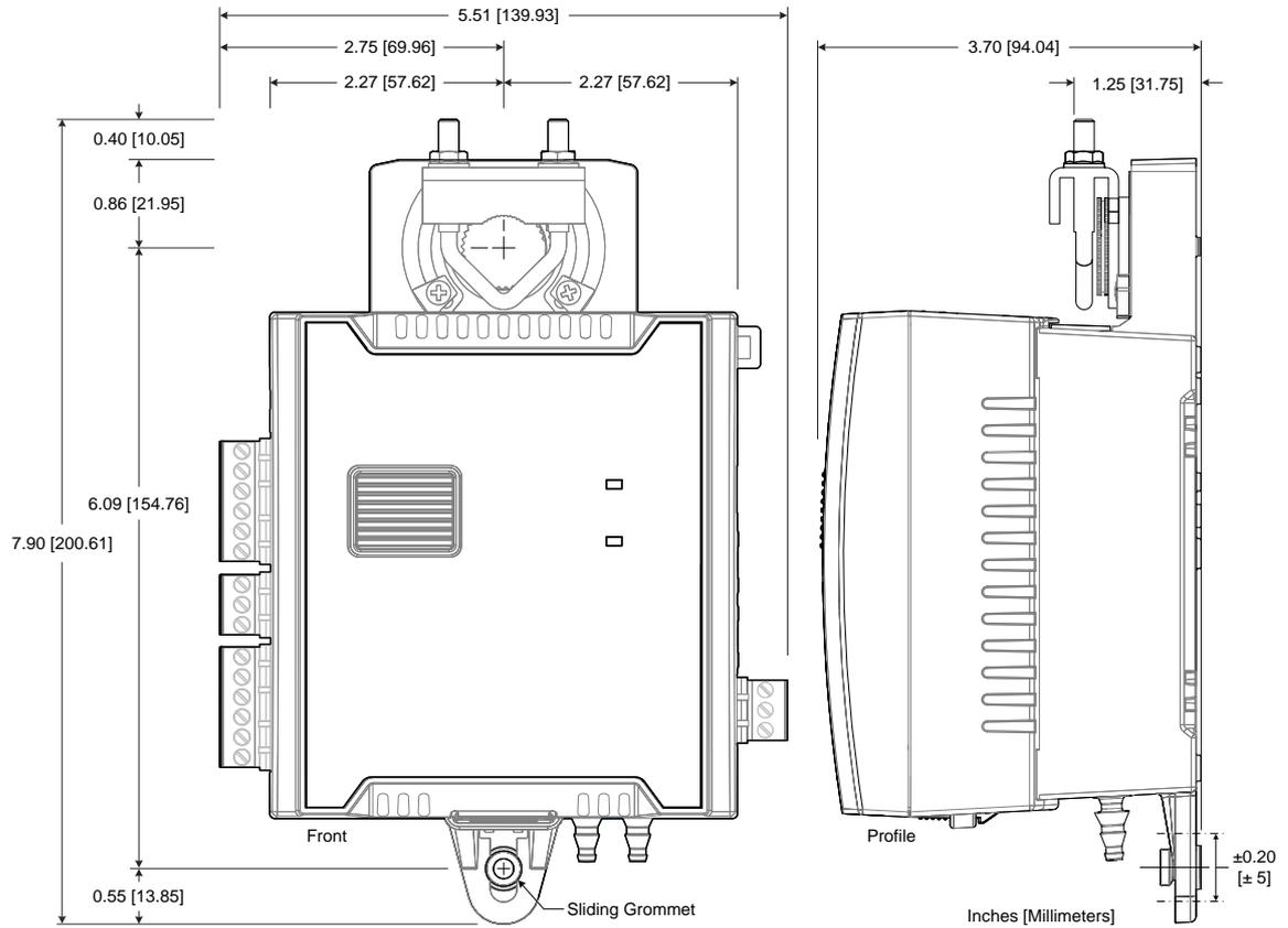
□ ECY-VAV-PoE Model (H × W × D) ——— 7.90 × 8.17 × 3.70" (200.61 × 207.59 × 94.04 mm)
