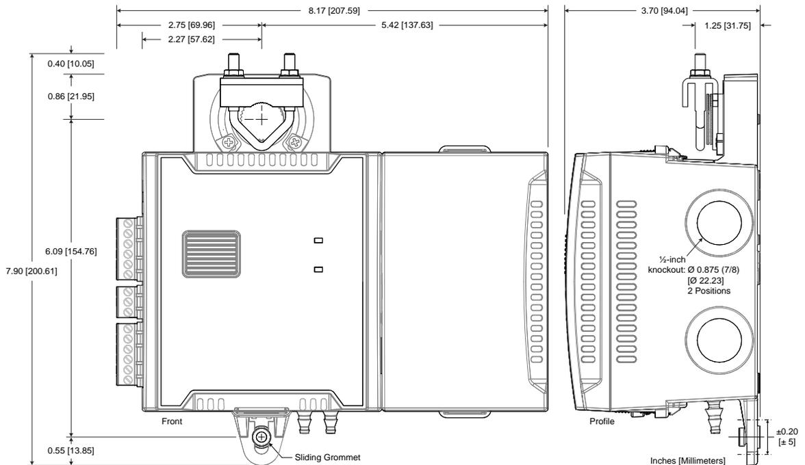
□ With Terminal Covers (H × W × D) ——— 7.90 × 10.84 × 3.70" (200.61 × 275.26 × 94.04 mm)
